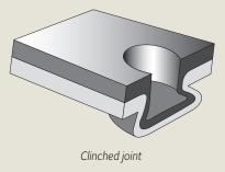
This process requires neither preformed holes nor additional material. Since the joint does not need to be heated, there is no heat-affected zone.
