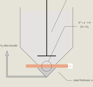
This test can only be used on steel with cavities, i.e. aluminiumkilled steel. In the case of IFS, susceptibility to "fish scale" defects is measured by means of an enamelling test in a moist atmosphere or by using a low-adhesive ground-coat enamel (sensitive ground coat).
