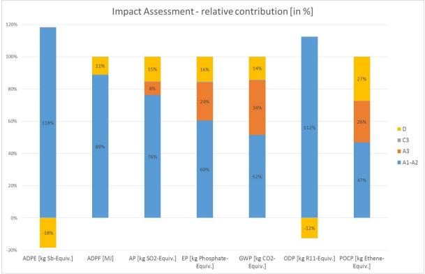
The graph above shows the relative contribution of the production stages (Module A1-A3), waste sorting and treatment (Module C3) and the benefits and loads beyond the product system boundary (Module D). For all the selected categories, the production stage (A1-3) provides the largest contribution to the results. Module D results in a noticeable potential benefit for Ozone Depletion Potential (**ODP**) and Abiotic Depletion Potential Elements (**ADPE**). Overall, C3 has a negligible contribution.
