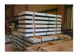
Corner RADIUS: most bars have corner radius within 9-20 mm.
