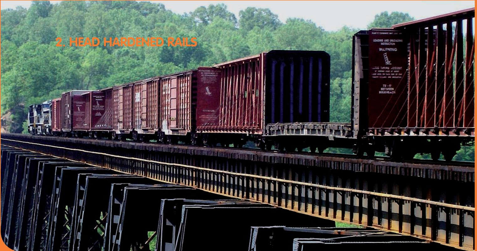
ArcelorMittal is the only producer in North America (Steelton) and after 3rd Quarter 2011 in Europa (Gijón), that has integrated in the rolling mill a head hardening system (HH), based on controlled cooling by water jets. More than one million tonnes of top-quality head-hardened rails have already been produced using this advanced technology.
