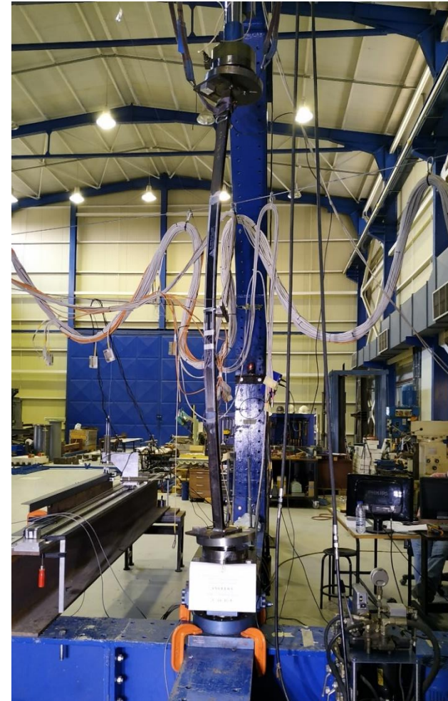
Buckling of the hybrid member
