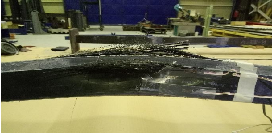
FRP under tension – fracture of the fibers
