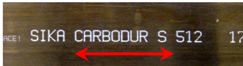
Uni-directional fibres orientation
