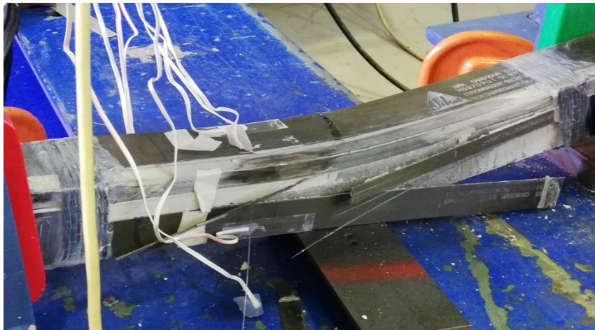
FRP under compression – plate breaking Detachment of the FRP plate due to shear strain
