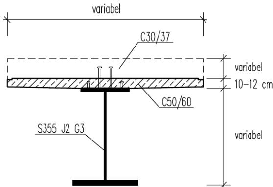
Fig. 1 – Typical cross-section of VFT®
