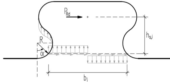
Fig. 19 – Forces and stresses in a critical section at ULS
