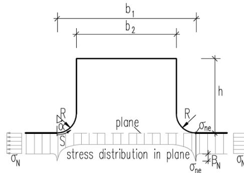
Fig. 16– Stress distribution due to notch effects
