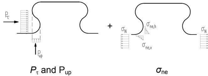
Fig. 12 – Forces on the steel dowel (PZ shape)
