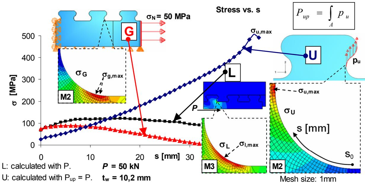
Fig. 17 – Stresses in steel dowel along arc length from specific actions:  $\sigma_{ne}$  ( $\sigma_g$ , G),  $P_\tau$  (L) and  $P_{up}$  (U)
