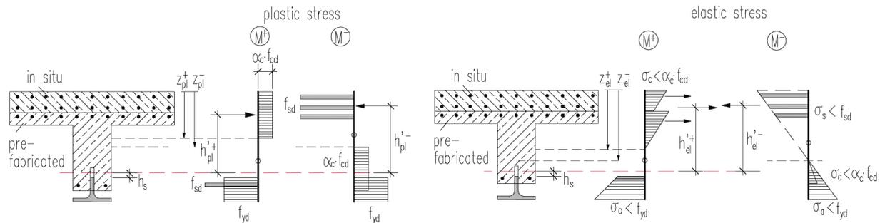
Fig. 14 – Determination of  $h'_i$  for ULS and SLS
