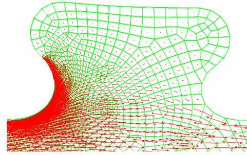
Fig. 21 – Principal stress trajectories in dowel ( $P_{Rd}$  and  $P_{up} \neq 0$  and  $\sigma_N$  influence)
