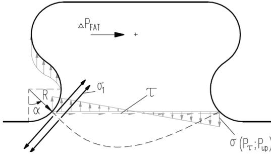
Fig. 20 – Analytic model for principle stresses (in dependency of the angular  $\alpha$ )
