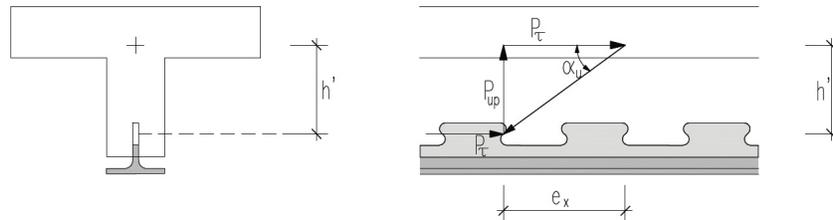
Fig. 13 – Uplifting force due to eccentricity of the shear joint to the neutral axis at support
