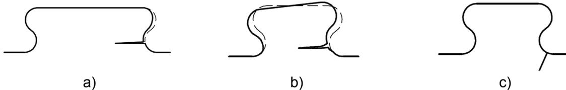
Fig. 8 – Failure modes for steel
