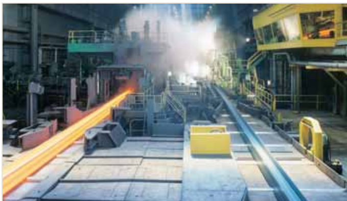
Rolled section entering QST bank (left)
