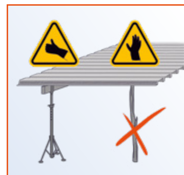
9 - Use a suitable prop equipment
