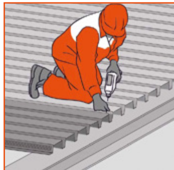
5 - Nail profiles in accordance with the installation progress
