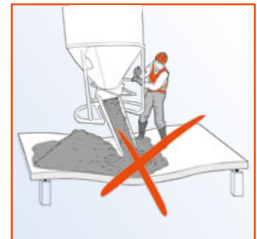
19 - Avoid any concrete accumulation while concreting
