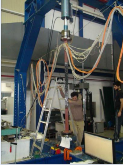
Fig. 3: Buckling tests on hybrid angle columns
