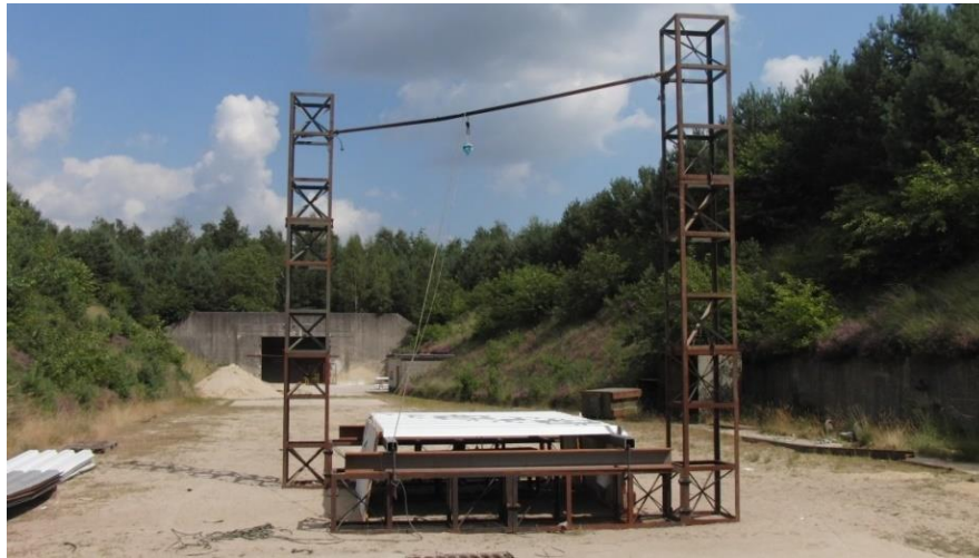
Figure 19: Positioning of the explosive, cladding test-setup
