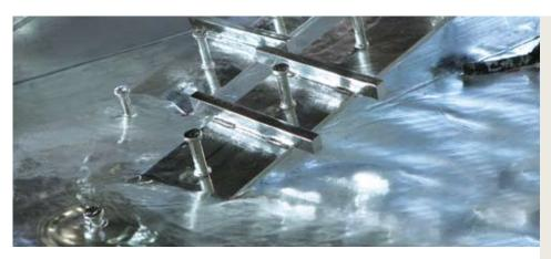
Nowadays, corrosion protection of steel car park structures is usually achieved by hotdip galvanization. During this process, rust and mill scale are removed from the surface of the beam in a pickling bath before immersion during 5–10 minutes in the bath of liquid zinc at 450 °C. Typically, a 150–250 µm thick zinc layer is formed which will protect the steel surface against atmospheric corrosion.
