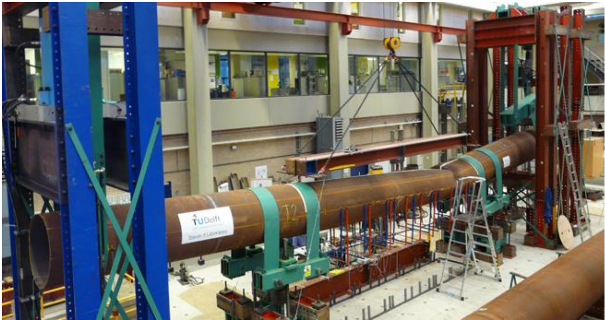
Figure 15 – Test rig in Delft in 4-point bending.
