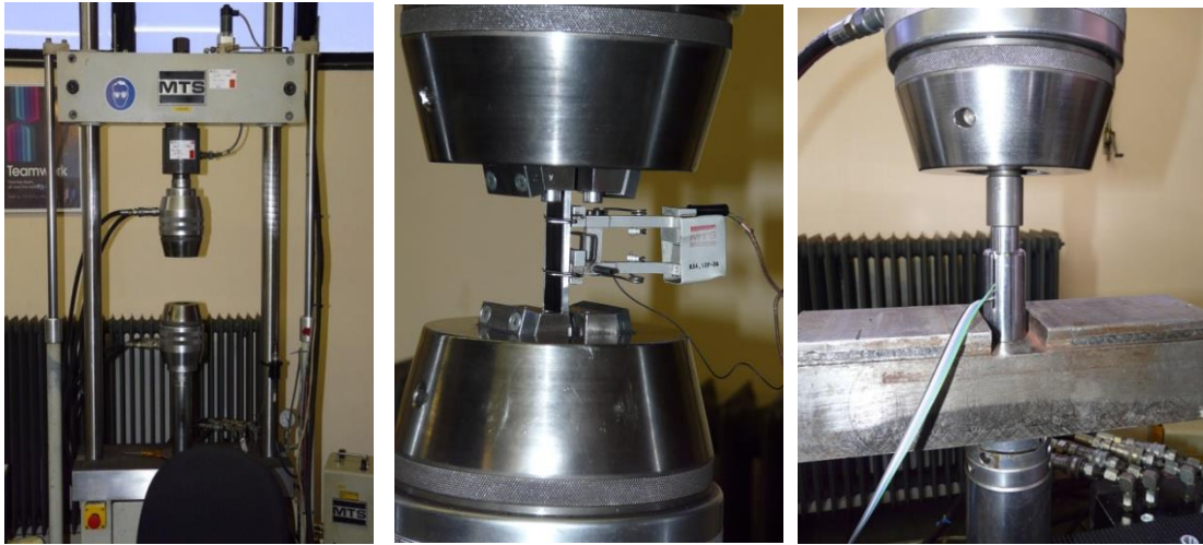
Figure 21 - Overview of tensile test setup (two figures left) and compressive setup by TU-Delft.
