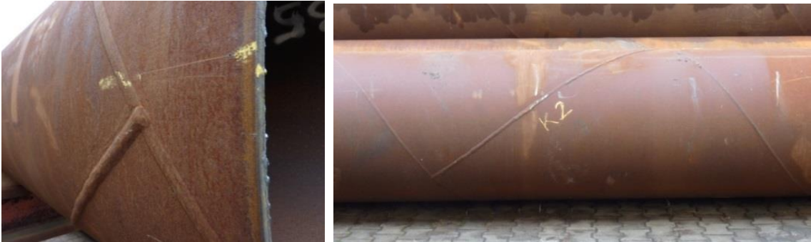
Figure 16 - K1: Coil weld at the end, K2: Coil weld in the centre.
