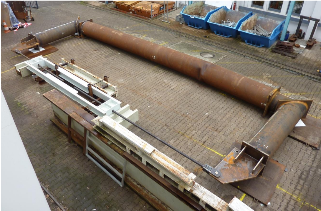
Figure 18 – Overview of test rig in Karlsruhe with buckled test K1.
