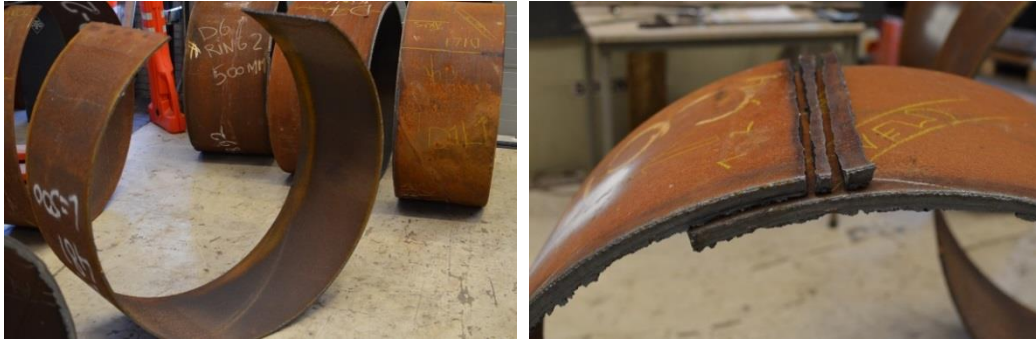
Figure 42 - Photos of cut rings Ring 481 (left) and D10R (right); since D10R appeared to close, more plate material was removed to let the ring freely deform.
