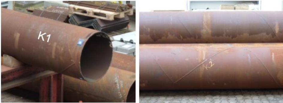
Figure 46 - Coil connection welds in specimens K1 and K2.
