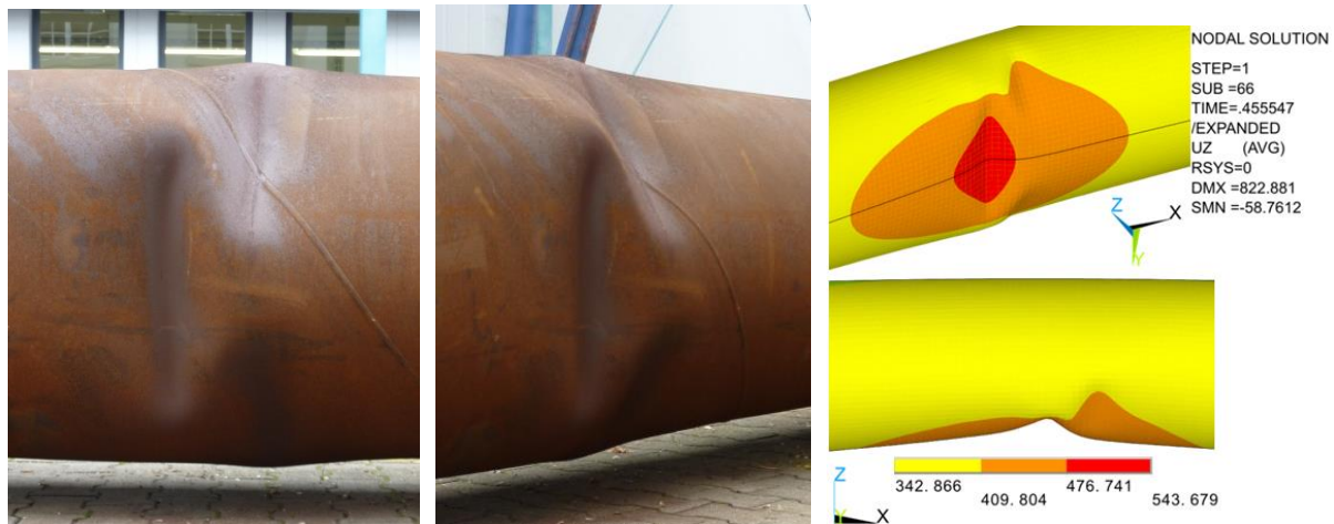
Figure 93 - K1 comparison with buckling mode simulation K1_C, geom. perfect, xz-symmetry only
