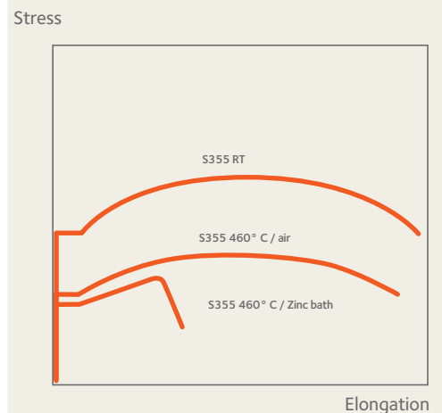
Figure 6 Schematic stress - strain diagram for structural steel S355 - comparison of the characteristics of S355 at room temperature (RT), at 460°C in the air, and during immersion in the zinc bath at 460°C
