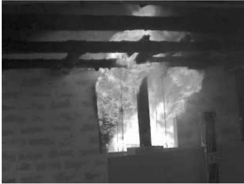
Figure 4 - CTICM Test 1: One column located in front of the opening - Facade view
