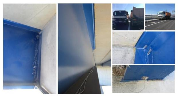
Figure 99 - Installed strain gauges on the section of the bridge in the in-situ test day
