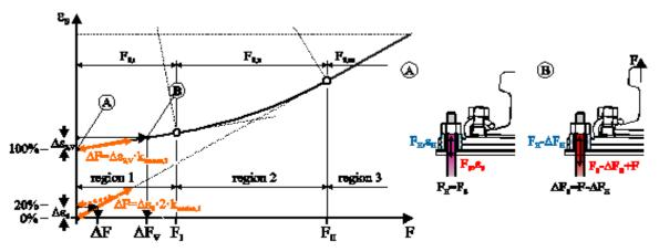
Figure 72 - Bolt force function: measured strain  $\Delta \varepsilon_s$  over jack force  $\Delta F$  at rail support point
