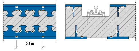
Figure 76 - Position of strain gauges
