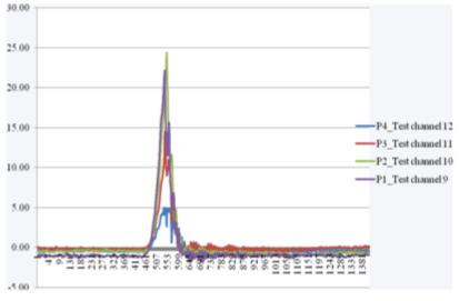
Figure 116 - "s<sub>din</sub>" values from test load schema 3 – LC3
