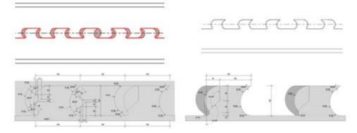
Figure 47 - Execution details of the steel girders, geometry of the steel dowel
