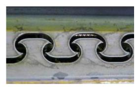
Figure 8 - Dowels after cutting-process
