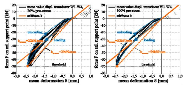
Figure 70 - Mean lowering / deformation of the ribbed base plate depending on the force applied (20% pre-stress, 100% pre-stress)
