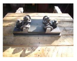
Figure 12 - Rail support before mounting
