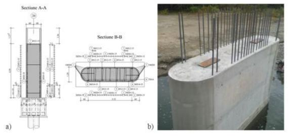
Figure 54 - Pier reinforcement plan (a), Site photo of the pier (b)
