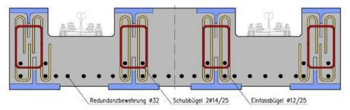
Figure 6 - Schematic reinforcement for the cross-section
