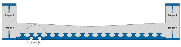
Figure 84 - Cross section VFT-Rail with composite dowels and composite slab
