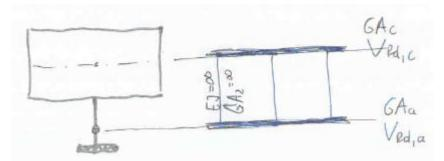
The point is how to dimension such sections for vertical shear, especially how to design stirrups in thick concrete plate. Reinforcing system is very safe in PE4 because aware of this idea we had to over dimension it – in future (if problem solved and design formulas established) a big reduction of stirrups can be expected for such structures. Important aspect of thick plate is big torsional stiffness what improves cooperation between girders.
