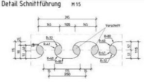
Figure 7 - Detailed cutting-geometry
