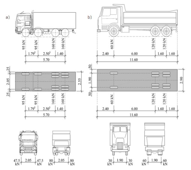
Figure 97 - a) A30 convoy – lateral view, plan view, front / back view; b) MAN TGA convoy – lateral view, plan view, front / back view.
