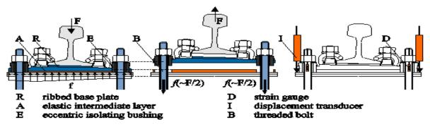
Figure 66 - Load bearing mechanism of rail support point ECF (principle, superelevated illustration), measurement equipment at rail support point ECF (principle)
