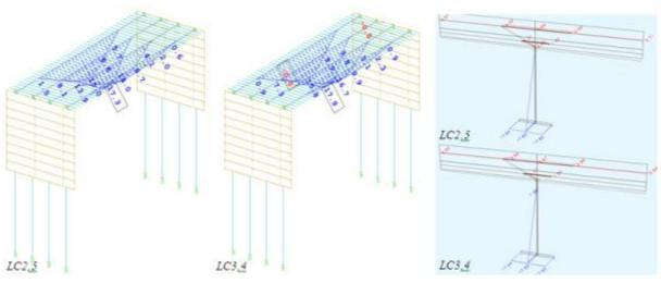
Figure 119 -  $_{,,s_{stat}}$  values from dynamic test load schema 3, 4 – LC3,4 (v = 50 km/h) and load schema 2 – LC2,5 (v = 30 km/h)
