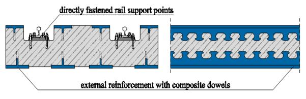
Figure 60 - Transverse cross section (left) VFT-Rail® with rail support points directly fastened to the superstructure and composite dowel and longitudinal cross section (right, depicting the clothoidal shape of the dowels)
