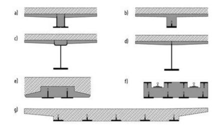
Figure 124 - VFT-WIB<sup>®</sup> section types a) to g) [4]
