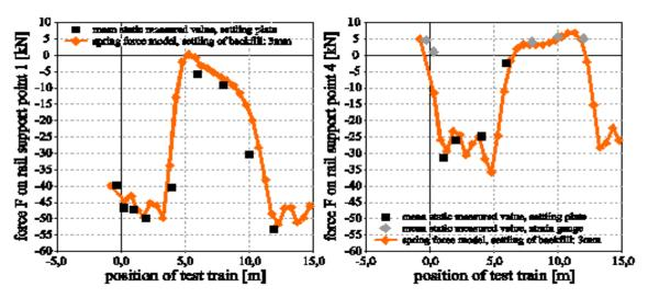
Figure 73 - Compression force / tension force acting on controlling rail support points 1 (left) and 4 (right), caused by static loading (test train)
