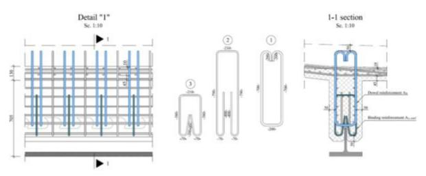
Figure 48 - Composite dowels – reinforcement details
