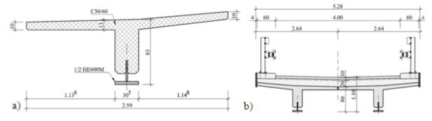
Figure 46 - VFT-WIB – mono-WIB cross section (a), Superstructure cross section (b)
