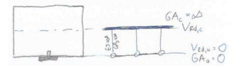
This is "general" composite section expressed by Vierendeel beam (vertical shear force is handled by steel and concrete parts acting together depending on their geometries and internal lever arm – see annex):
