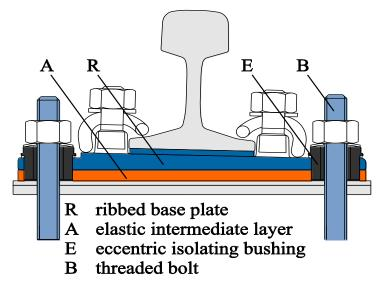
Figure 62 - Structure rail support point ECF [ThyssenKrupp 2006]
