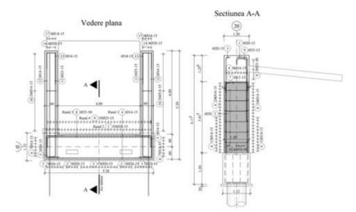
Figure 52 - Abutment reinforcement plan
