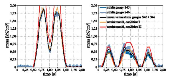
Figure 82 - Stresses in lower flange caused by crossing of test train (100 km/h, left) and regional train (120 km/h, right)
