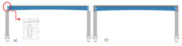
Figure 106 - Construction stages: a) Simple supported girder; b) Frame effect
