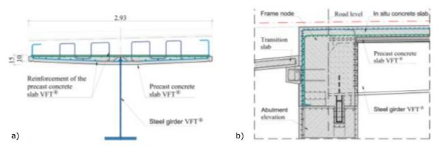
Figure 92- a) Reinforced cross section of the Prefabricated Composite Girder VFT<sup>®</sup>, b) Frame node reinforcement detail
