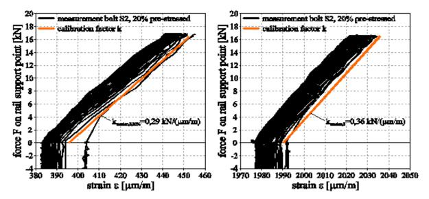
Figure 71 - Strain change in measurement bolt S2 depending on applied force (20% pre-stressed, 100% pre-stressed)
