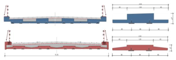
Figure 41 - General new cross sections and details with the precast elements
