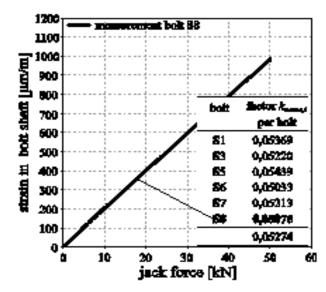
Figure 68 - Calibration of measurement bolts (here: measurement bolt S8), conversion of strain in measurement bolts into pre-tension force
