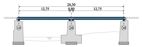
Figure 61 - Longitudinal section railway crossing over the river "Simmerbach" with two VFT-Rail® girders, placed on toughened sub-structure
