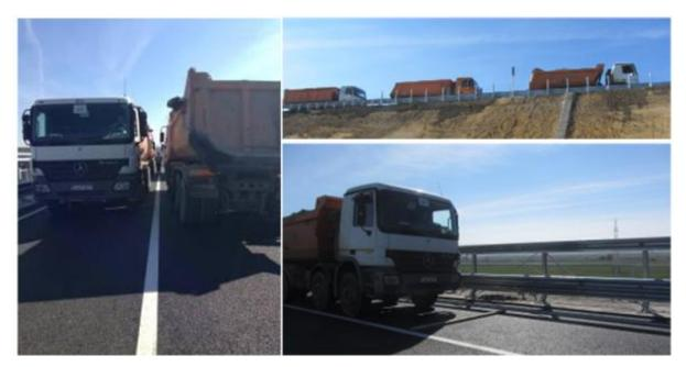
Figure 98 - MAN TGA convoy - front view, lateral view; dynamic load test MAN TGA vehicle.
