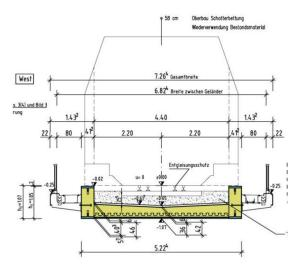
Figure 131 - Leuna Bridge: Cross section
