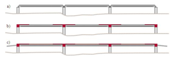
Figure 49 - Superstructure construction phases: laying of the VFT-WIB composite girders in their final position (a), frame node and end sections of the deck concreting (b), deck concreting (c)
