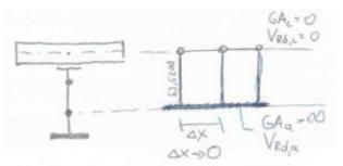
This is classic concrete section expressed by Vierendeel beam (concrete part alone takes vertical shear force):
