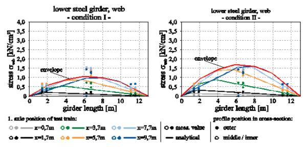
Figure 80 - Measured strains / stresses at web of lower external reinforcement, compared to calculated values for condition I (left) and condition II (right)
