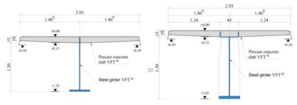
Figure 91 - The formwork cross section of the Prefabricated Composite Girder VFT®
