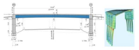
Figure 89 - Left: longitudinal section, Right: design model
