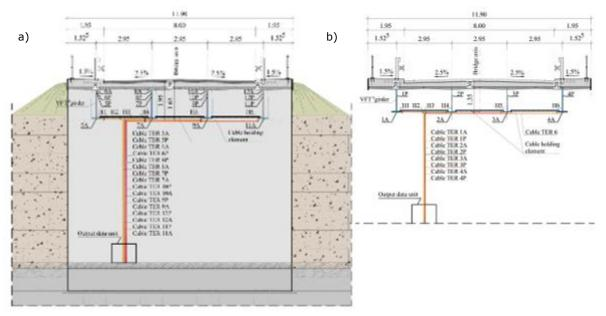
*Figure 101 - Installed strains on the section of the bridge; a) Cross section on the supports area; b) Cross section on the field.*
