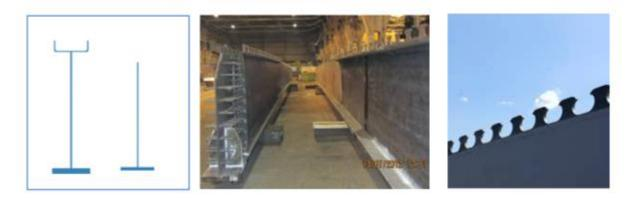
*Figure 94 - The steel girder type sections; Steel girders in the workshop; the cutting line geometry of the composite dowels.*
