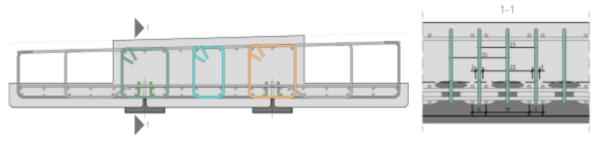
Figure 42 - Reinforcement detail of the precast composite girder
