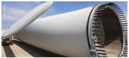
figure 10: Connection for wings
