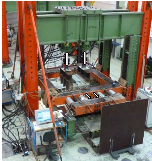
Figure 5-12. Test set-up horizontally lying studs under transversal fatigue load in cracked concrete.
