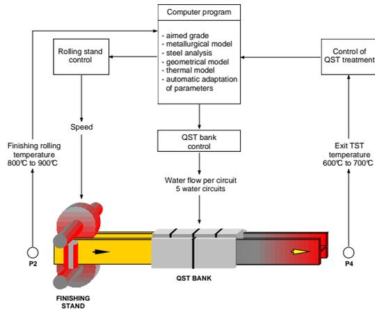
Figure 7 – Control of a QST process to produce a beam in an aimed grade
