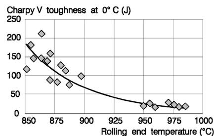
Figure 3 – Influence of the rolling scheme on toughness of silicon killed EAF steels
