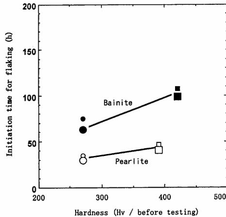
Figure 20 – Initiation time for RCF damage as a function of hardness
