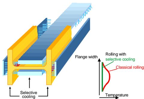
Figure 8 - Influence of selective cooling during rolling on the temperature profile of the flange width
