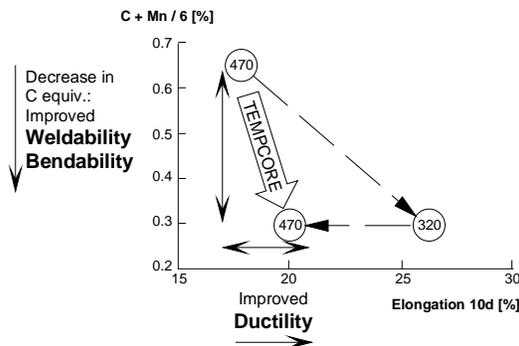
Figure 16 – Weldability and ductility properties of Tempcore rebars
