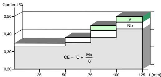
Figure 4 – Steel alloying contents for S355, controlled rolling
