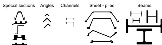
Figure 1 – Hot rolled sections
