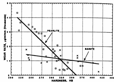
Figure 19 – Wear rates vs. hardness for pearlitic rail steels (open square) and bainitic steels
