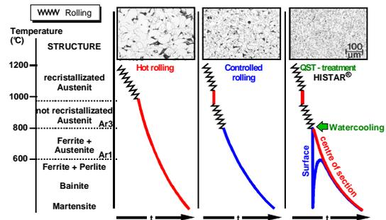
Figure 9 - Comparison of the different rolling process for beams
