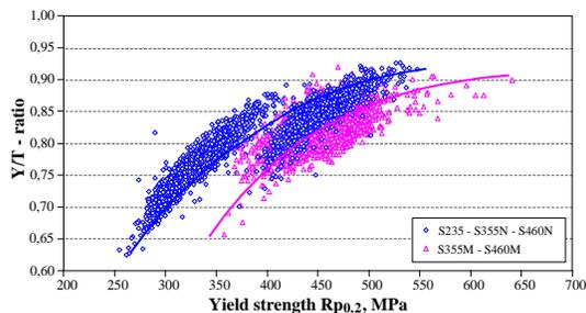
Figure 12 – Re/Rm ratio in function of the yield strength and rolling process
