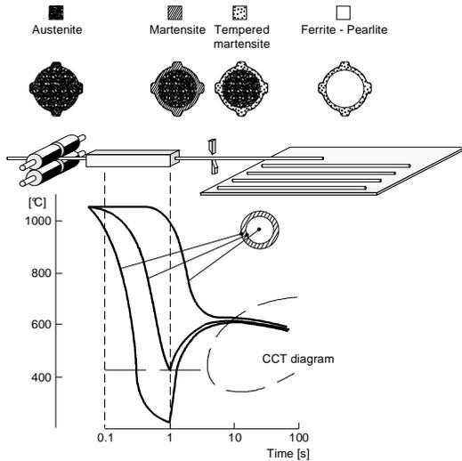
Figure 15 – Tempcore process and relationship with CCT diagram
