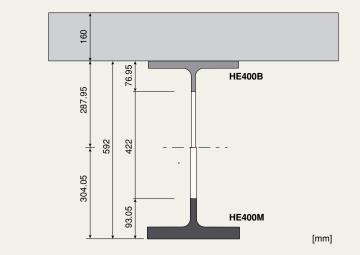
For the main beams (span of 16.8 m) ACB/HEM400/HEB400 profiles in steel S460 have been used, see Figure 19. The main beams with the shorter span of 4.2 m are ACB/HEM360 in S460.
