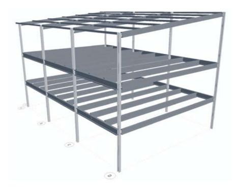
The slab is a composite plate of 15 cm total thickness with steel sheets COFRASTRA 70, Figure 23.
