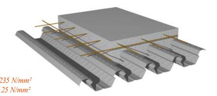
• Steel S235:  $E_s = 210000 \text{ N/mm^2}, \quad f_y = 235 \text{ N/mm^2}$ • Concrete C25/30:  $E_{cm} = 31000 \text{ N/mm^2}, \quad f_{ck} = 25 \text{ N/mm^2}$
