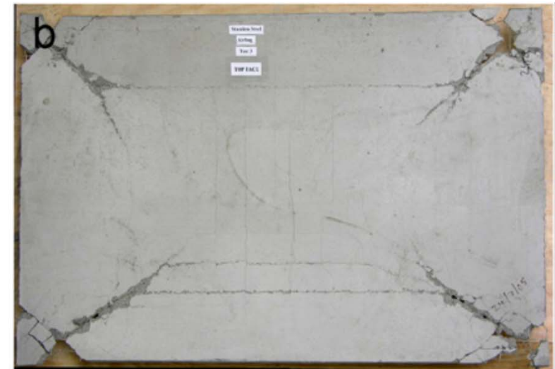
Compressive failure of concrete
